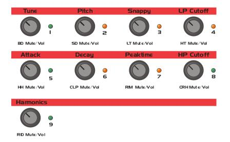
At any time and in any mode, you can mute the instruments by clicking on one of the displayed encoders 1-9. When the instrument is muted, the corresponding LEDs blinks red.
