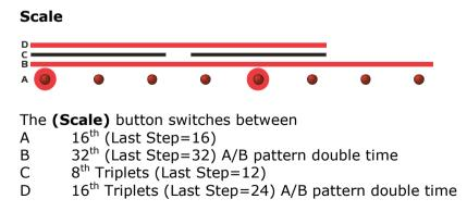
The **(Scale Bars)** that are printed above the **(Step LEDs)** indicate where the quarter downbeats of the selected scale are.
